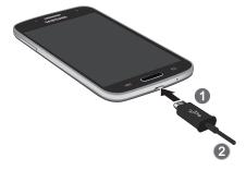
**2.** When charging is finished, remove the flat end from the interface connector jack on the phone.
