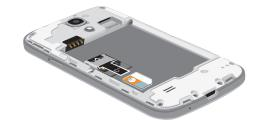
Note: If the card is not inserted correctly, the phone will not detect the SIM card. Re-orient the card back into the slot, if the SIM is not detected.
