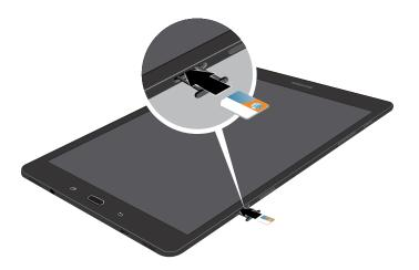
**Caution**: Exercise care when using the metallic removal tool to eject the internal SIM card slot.
