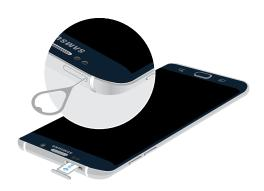
**Caution**: Exercise care when using the removal tool to eject the internal SIM card slot.
