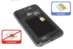
Note: If the card is not inserted correctly, the phone will not detect the SIM card. Re-orient the card back into the slot if the SIM is not detected.
