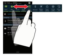
The following functions (default) can either be activated (green) or deactivated (gray): Wi-Fi, GPS, Sound, Screen rotation, Multi window, Bluetooth, Airplane mode, Power saving, Driving mode, and AllShare Cast.
