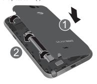
Press along the edge of the back cover (3) until you have a secure seal.
