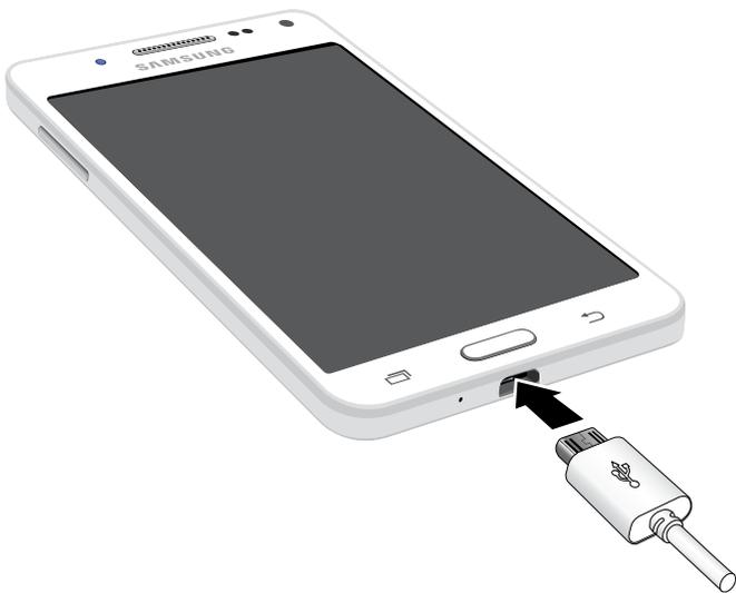
1. Insert the USB cable into the port.
