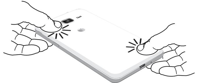
1. Place the back cover onto the back of the device and press down.
