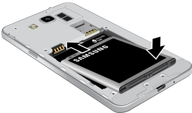
1. Insert the battery into the opening on the back of the phone, making sure the connectors align.
