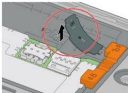
3. Insert the microSD card into the microSD card holder with the gold contacts facing down. Gently push the card in until it snaps into place.
