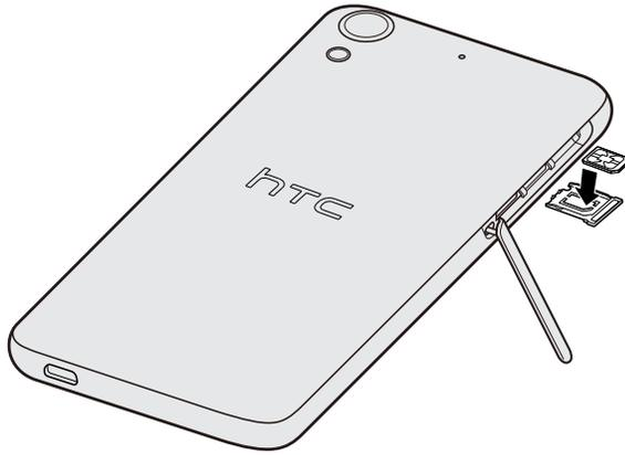
5. When reinserting the tray, make sure it is facing up so that the nano SIM card doesn't fall out. Slide the tray all the way into the slot.
