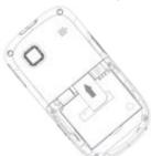
4 Reinsert the battery and replace the back cover.
