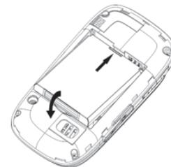
**Caution:** Make sure the cover is lined up before pressing it into place. Do not force it. Doing so will damage the back cover.
