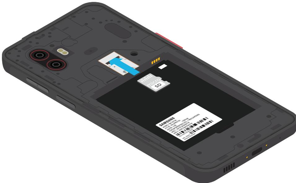
5. Insert the battery into the opening on the back of the device, making sure the connectors align. Gently press down to secure the battery.
