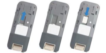
1. Open the protective door by pressing on the cover with and sliding the door off.
