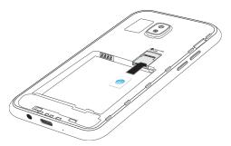
Slide the memory card into the slot with the gold contacts facing down.
