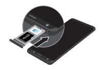
4. Slide the SIM card/Memory card tray back into the slot.
