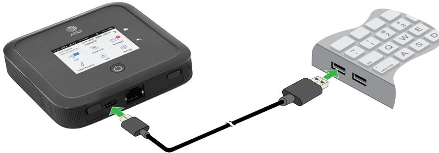
The Battery icon on the LCD indicates that the battery is charging.
